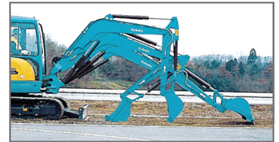
Load-sensing Hydraulic System
